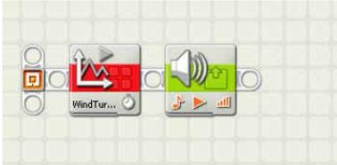
Above is a screenshot from the data logging program Wind Turbine 1 included in the zip folder. This program collects data from the Energy Meter and has a stop tone when the data logging experiment ends.
