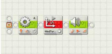
Above is a screenshot from the data logging program Wind Turbine 2 included in the zip folder. This program collects data from the Energy Meter, turns the tower 45 degrees and has a stop tone when the data logging experiment ends.
